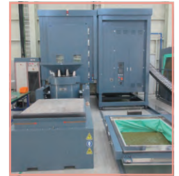
고변위복합환경진동시험기 Long-stroke shaker for large payload & Climate environmental chamber
