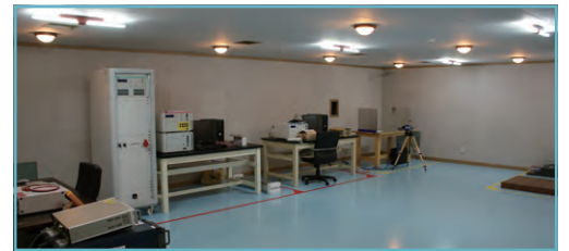
전자파 차폐실 Electromagnetic shielded room
