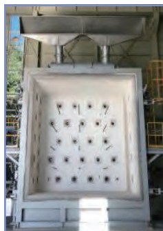
조선해양 기계류 3면 입체가열로 Three-sided heating furnace for shipbuilding and marine machinery
