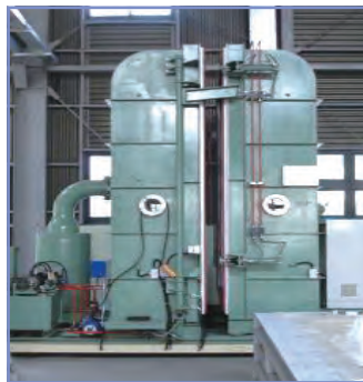
차연성시험장치 Smoke control test equipment
