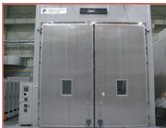
복합환경 (고온, 저온, 습도) 구현 Walk-in 챔버 Walk-in chamber for implementation of complex environment (High temperature, low temperature, humidity)
