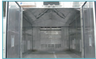
염수분무 시험기 Salt spray tester (S0.6*0.6*0.3, M2*1.5*1.5, XL5*7*5m)
